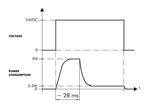
Speed-up valves have very high capacities and fast response times, despite very low power consumption. When a command is received, a high power is generated for a brief period of time so that the valve switches rapidly. Position maintenance power is then delivered, being about one tenth the former value. This solution also allows very low valve temperatures.
