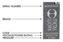
Despite its small size, each PLT-10 is laser-marked with the main data. The serial number incorporates the date of manufacture, the production lot and the test data. This allows full traceability of the valve and its components.
